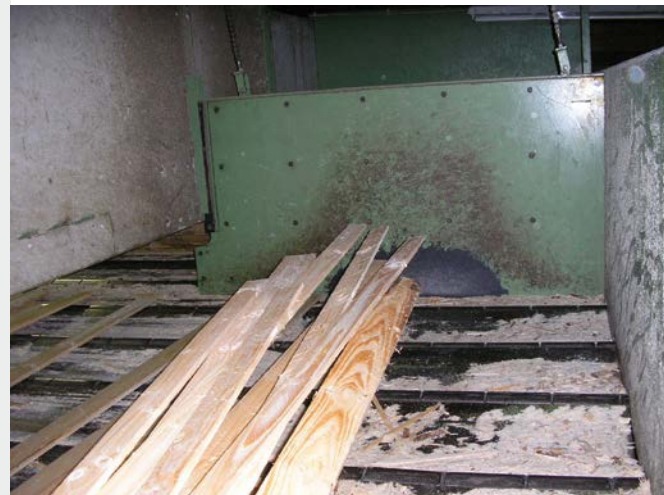
Impact protection for wooden battens
