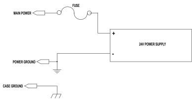
Figure 6-10: ACS Drive/Controller Single Supply – Main Power
