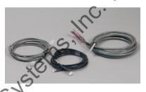
Tolomatic offers a motor power cable with drive and motor mating connectors, an encoder cable with drive and encoder connectors, and an I/O cable with drive mating connector to flying leads. Cables are available in either 3-meter or 5-meter lengths.
