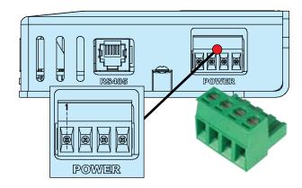
Figure 5-7: Input Power Connection
