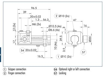
The universal intermediate jaw allows fast tool-free and reliable plugging and shifting of top jaws at the gripper.
