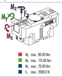
The indicated moments and forces are static values, apply per base jaw and may occur simultaneously. My may arise in addition to the moment generated by the gripping force itself. If the max. permitted finger weight is exceeded, it is imperative to throttle the air pressure so that the jaw movement occurs without any hitting or bouncing. Service life may be reduced.
