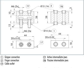
Force measuring jaws measure gripping forces, but can also determine workpiece weights or dimensional deviations. There are active and passive intermediate jaws (FMS-ZBA or FMS-ZBP). At least one active force measuring jaw is required per gripper, the rest can be passive. For each active jaw, a FMS-A1 control unit and a FMS-A connection cable are required.
