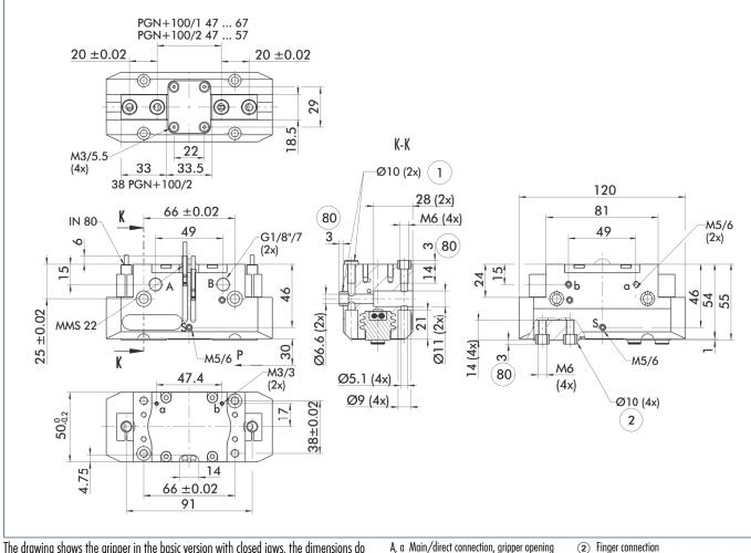
The drawing shows the gripper in the basic version with closed jaws, the dimensions do not include the options described below.
