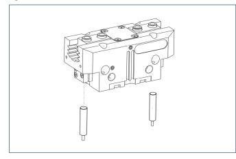
End position monitoring mounted with mounting kit
