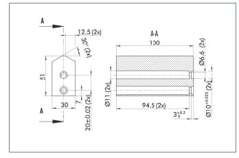
Finger blanks for customized subsequent machining
