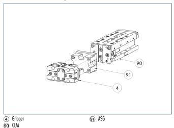
This gripper can be combined with the standard linear modules LM, KLM, CLM and ELM of the GEMOTEC modular system. For more information see our main catalog "Modular Assembly Automation".
