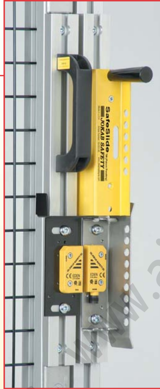
With the door closed and SafeSlide engaged, the Eden Adam and Eva are able to make contact and the door is secured.
