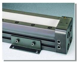
For intermediate support, tube support brackets can be mounted to the BC3 model. Made of black-anodized aluminum, the brackets are attached to the bottom and sides of the cylinder tube with rail nuts. The number of tube support brackets required and their placement depends on the overall length of the BC3 model and the load weight being moved and supported. Refer to the tube support data chart below.
