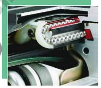
Patented Wedge\*\* guarantees that the raceways are parallel which insures a preload that is consistent throughout the length of the cylinder.
