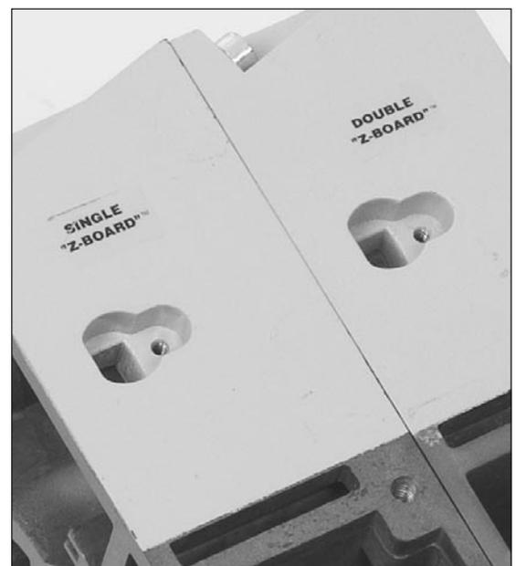
Label on manifold block indicates installed---"Z-Board"™ type.
