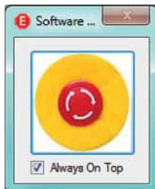
Figure 4-3: Software Emergency Stop
