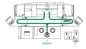
Two-pressure selector used for multi-pressure applications.
