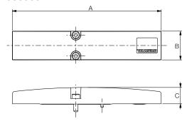
Used to block off a manifold station block for future use
