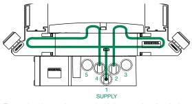
External outlet regulator used with jumper plate for single or dual pressure.
