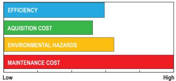
Hydraulic systems can be higher to operate because of the continual power required to maintain pressure. They also require high levels of maintenance and are subject to performance issues when fluctuating temperatures affect oil viscosity.
