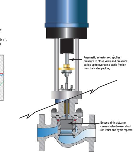
Pneumatic slip stick is caused from excess air build up in the actuator to compensate for encountered static friction from valve packing materials and components and causes the valve to overshoot the set point resulting in fluctuating valve performance.
