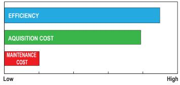
Unlike brush motors, servo motors have no brushes to wear and can operate at 100% duty cycle with little to no maintenance. They offer closed loop feedback with high resolution, accuracy, repeatability and precise control. Although they have a higher acquisition cost, they provide the best performance and quick response times, crucial in many valve applications.
