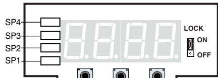
0.56" LED Display Board - Front View
